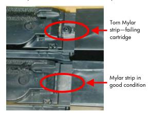
Print cartridge Mylar strip in poor and good condition
